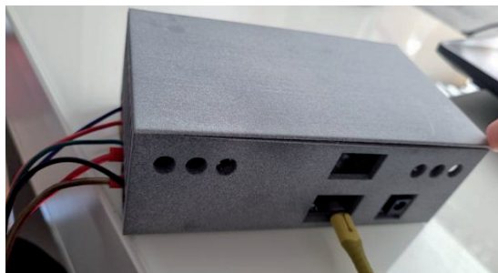
Figure 2: Acknowledgments3D-printed enclosure with ventilation openings and slots for sensor cables and switch access.
