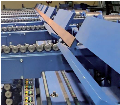
Figure 5: Photo of a fragment of a machine positioning a flat bar for measuring straightness.
