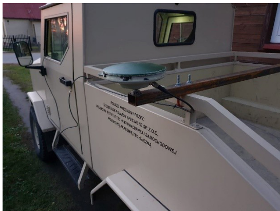
Figure 2: View of installed antennas of GNSS system
