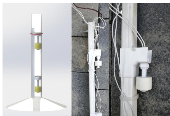
Figure 9: Mounting of sensors inside the cylinder.
