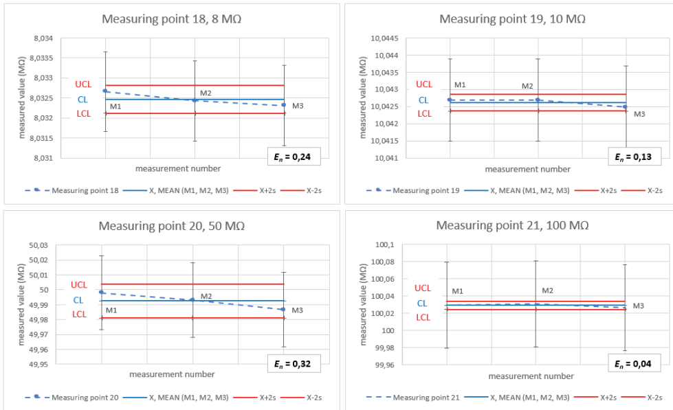
Figure 1 Example of evaluation of stability of resistance decade at selected measuring points
