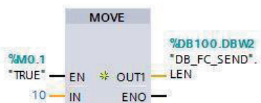
Fig. 11: Configuration of input LEN in TSEND_C block.
