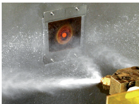
Fig. 3: Directly heated probe of the physical model.
