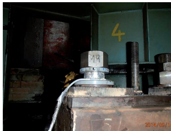
Fig. 12: View to dynamometer installed on anchor bolt of casting pedestal.
