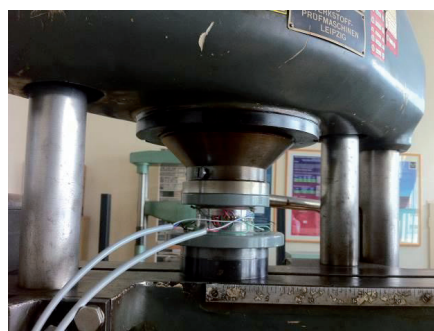
Fig. 8: Compression of dynamometer in test machine.
