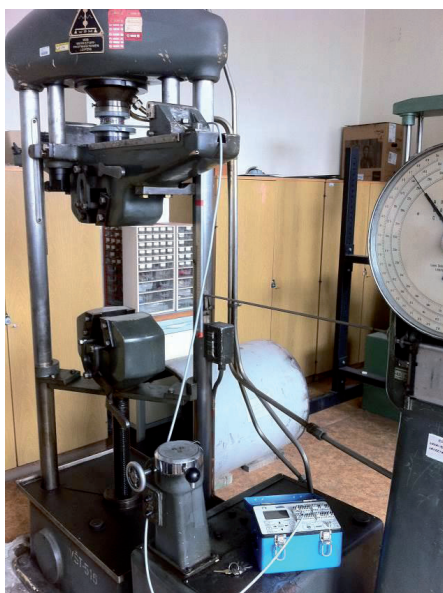
Fig. 6: Measurement chain for calibration of dynamometers.
