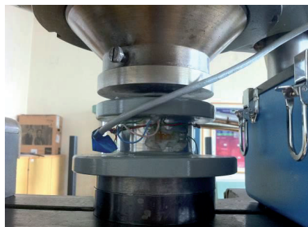
Fig. 7: Dynamometer inside of tension grips of test machine.
