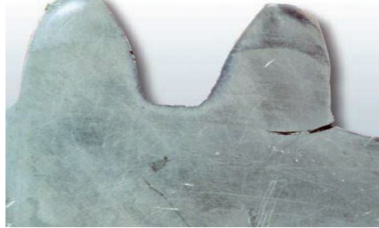
Fig. 5: Crack growth through the gear tooth
