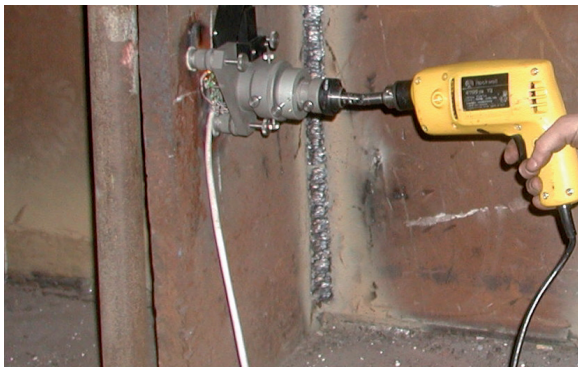
Fig. 10: Hole-drilling by systém RS 200.
