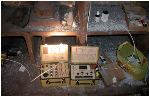
Fig. 11: Strain-gage apparatus P 3500 with switching box SB 10.
