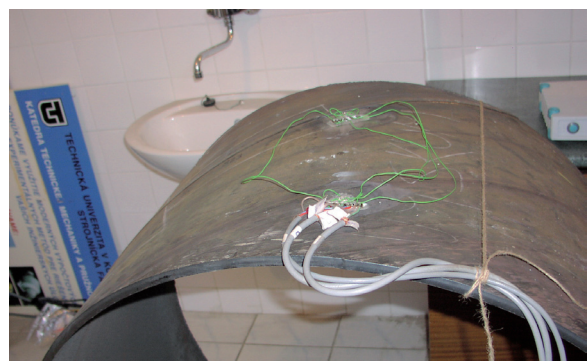
Fig. 6: Strain-gage RY 61 on the pipe.
