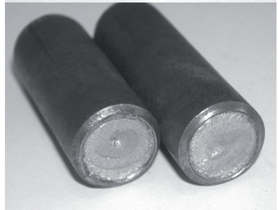
Fig. 4 C45 steel grade elements obtained during wasteless splitting process at: \alpha=45^\circ , \Delta r=2 mm, \theta=2^\circ (upper figure) or \theta=3^\circ (bottom figure)
