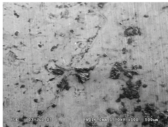
Fig. 7 Surface of sintered Co-Cr-Mo, mag. x100
