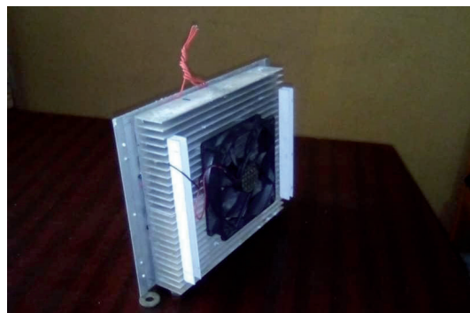
Figure 5: Assembly of Receiver plate, modules heat sink and cooling fan
