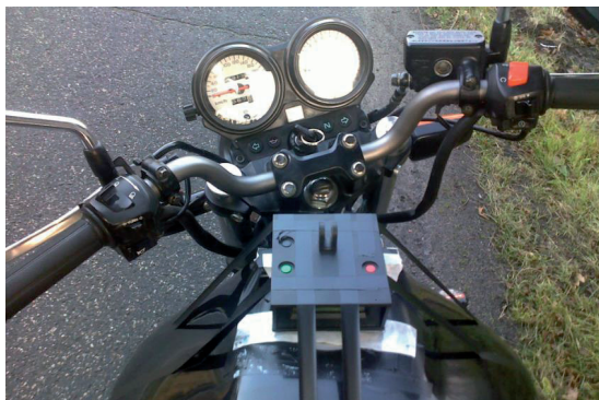
Fig. 2: Method of mounting the measuring device on a motorcycle.
