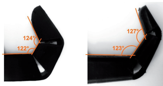
Figure 7: Physiological model in flexion (left), extension model in flexion (right).
