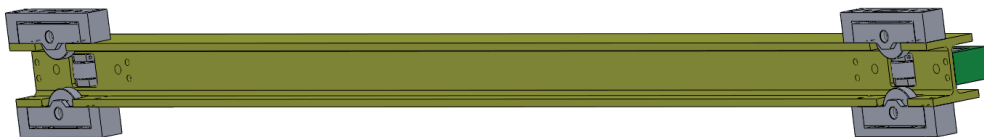
Fig. 9: HEM 180 with sprung guide wheels.
